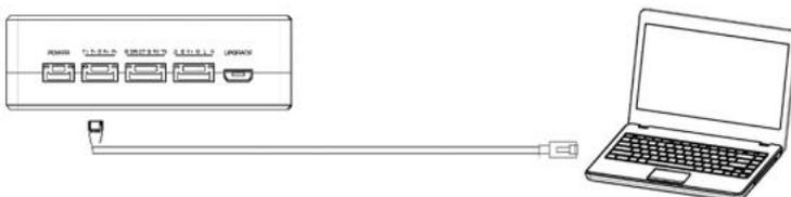
Ground unit has one way of outputting received video, to a PC or laptop.
