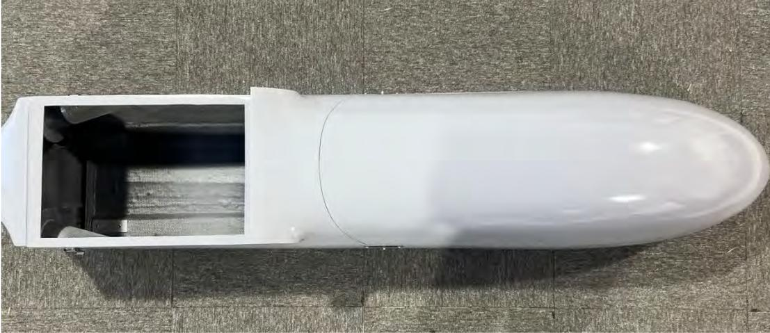
Center Wing: Connects power arms, ailerons, fuselage, and installs power and signal lines.
