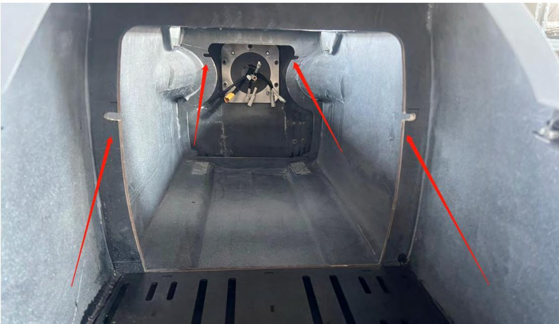
Install the fuel tank mounting nuts. Before making the openings, it is necessary to determine the positions of the nuts and then proceed with drilling as shown in the figure.
