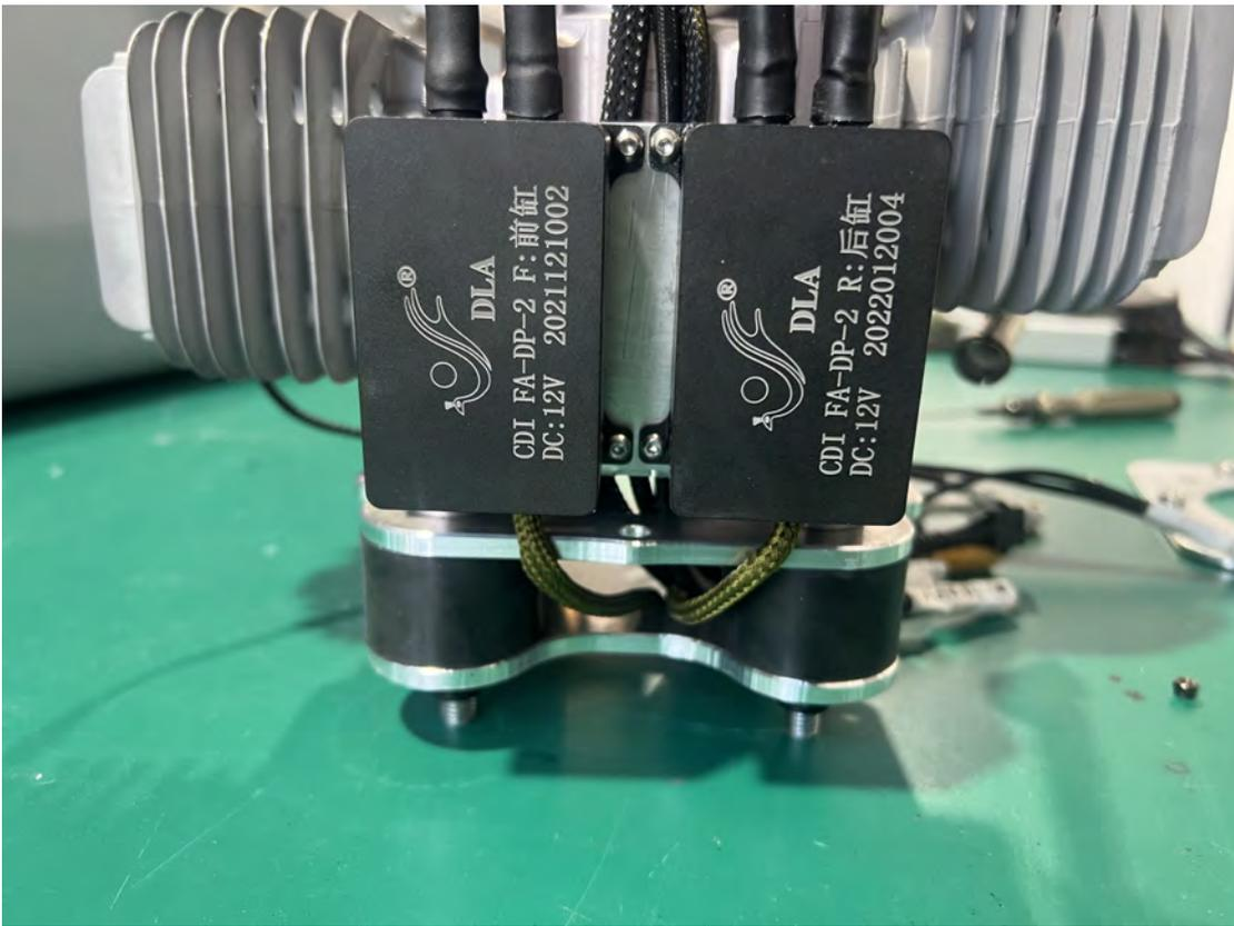
Secure the engine to the fuselage as shown in the figure.
