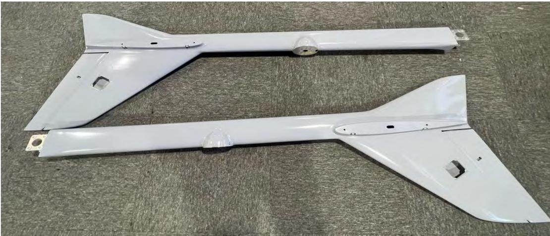
Horizontal Stabilizer: Installs elevator servos and servo reversers.
