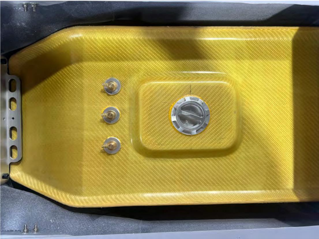
Install the front equipment board. Before installation, it is necessary to make positioning holes and limit holes as shown in the figure.
