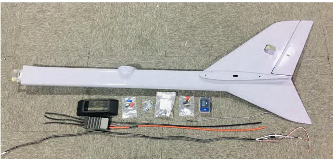
Install the motor, ESC (Electronic Speed Controller), servo, LED, and wiring as shown in the figure.
