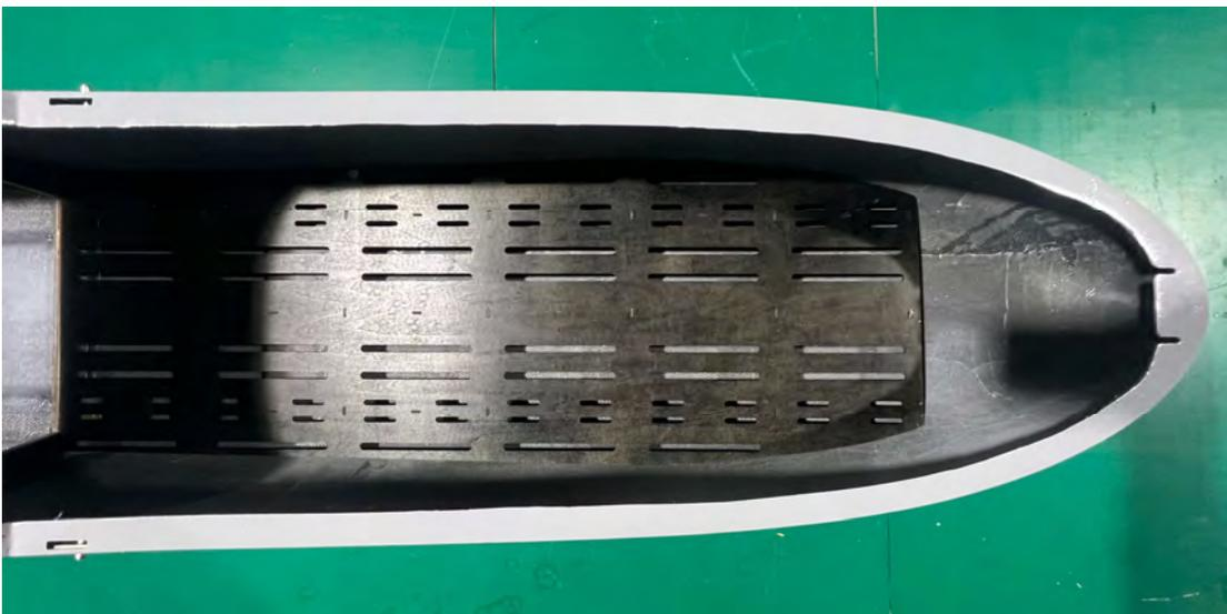
Installation of the airspeed tube holder. It is necessary to make openings during installation as shown in the figure.
