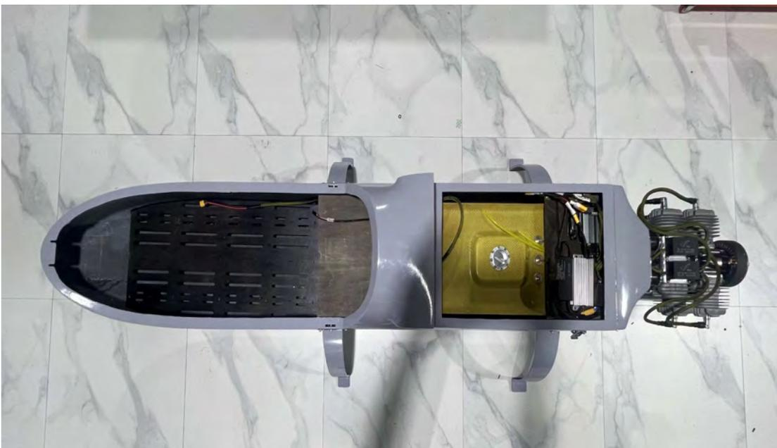
Installation of the wiring for the center wing and installation of the servo in the center wing compartment.
