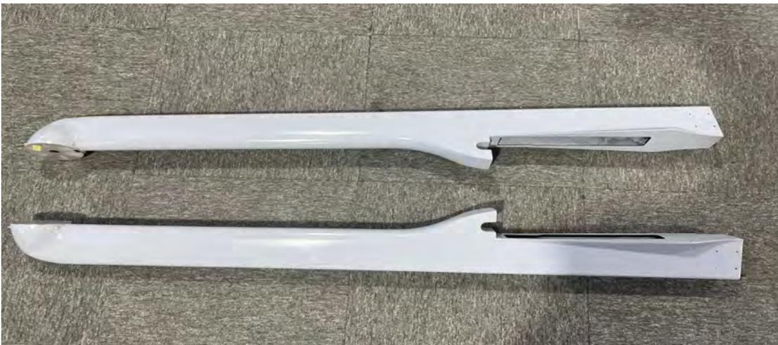
Rear Power Arm: Install vertical motors, electronic speed controllers, rudder servos, navigation lights, etc.
