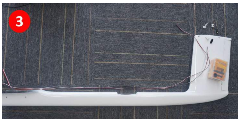
Picture 3 shows the layout of the wiring before servo installation.
