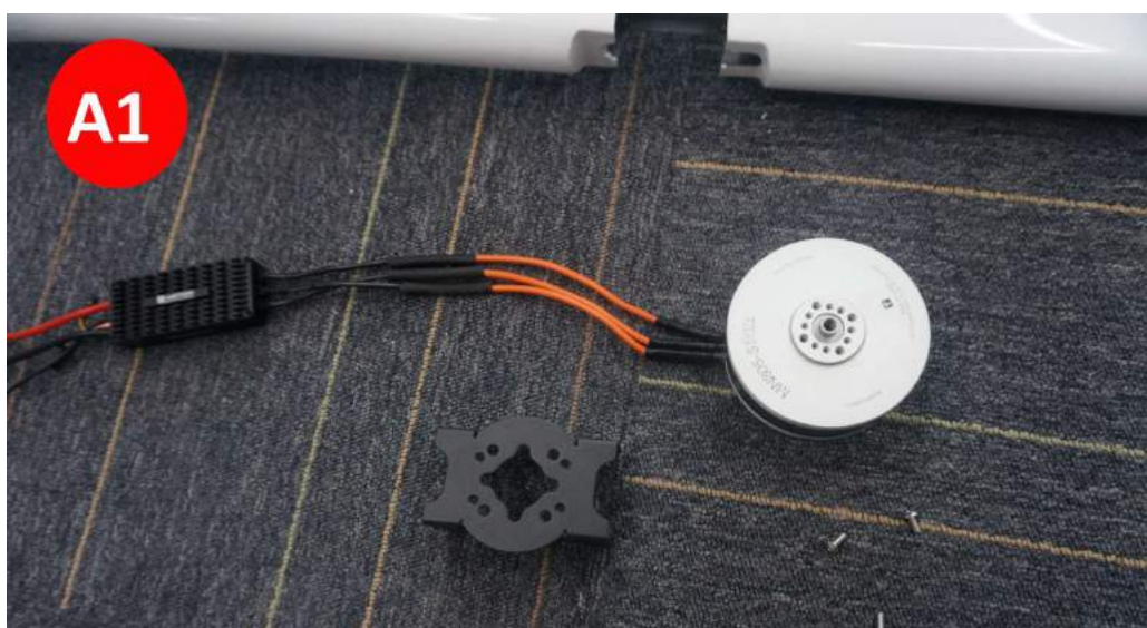
Picture 6(A1): Connect the motor to ESC (A1), ESCs to power extension wires, install extension wires for servo.(A2)
