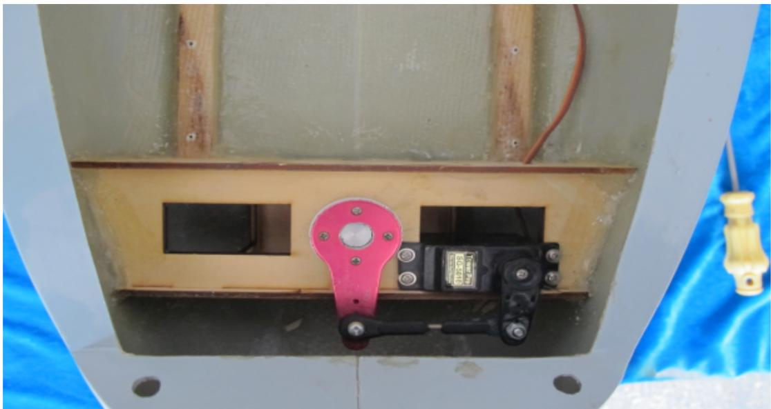
Install servo for nose gear
