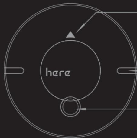
1.Ensure arrow points to front mounting direction of vehicle when mounting GPS to vehicle.
