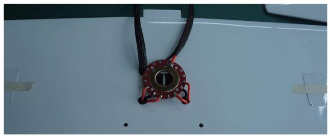
STEP Pay attention not to reverse the polarity of the positive and ground wires.
