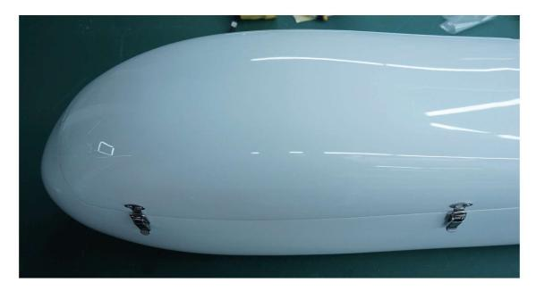
Tip: When drilling the hole for the pitot tube, place mount inside fuselage a drill from inside to the outside.
