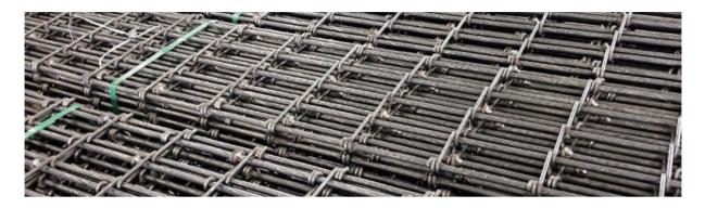
Osro rod straps are used in mining and tunnelling to provide continuous strip support between rock bolts, inhibiting fall-outs between the bolts and helping to maintain the integrity of the rockmass. The rock bolts are installed through the Osro straps and tightened against the rock surface.
