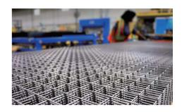
The manufacture of welded wire mesh includes threading spools of wire through a welding machine that is programmed to uniformly weld the many intersections of wire simultaneously, efficiently, and quickly.
